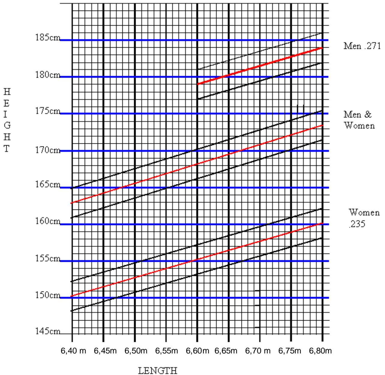
Instructions: For any particular ramp setting, a combination of HEIGHT at the top edge and LENGTH out of the water enclosed within the solid line is allowable. A combination that lies on the dotted (middle) line is the most desirable.
