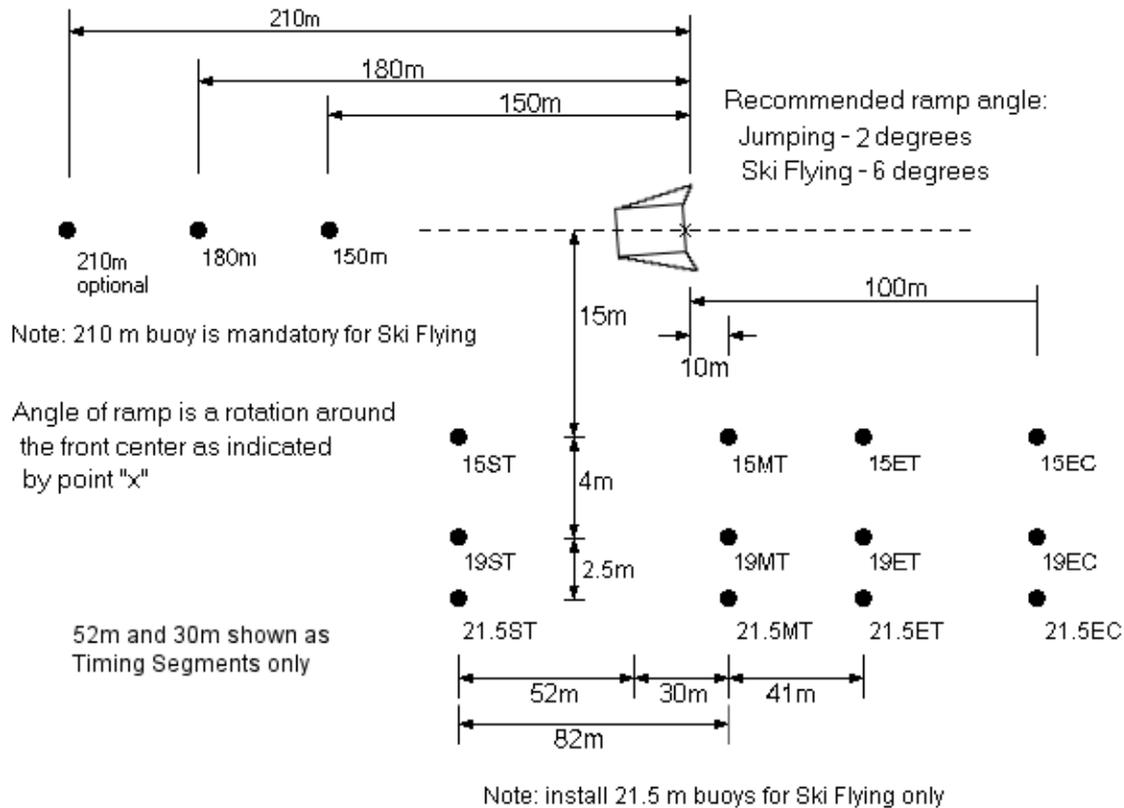
The ramp must be parallel to the jump course and slightly open. The tolerance for standard jumping is between +1.00° and +2.50° open.
